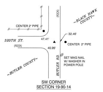
FND MAG NAIL IN 2" PIPE 8" DEEP. USING INFORMATION OBTAINED FROM CORNER CERTIFICATE NO. 2003-17458 IN THE OFFICE OF THE RECORDER, BLACK HAWK COUNTY, IOWA.
