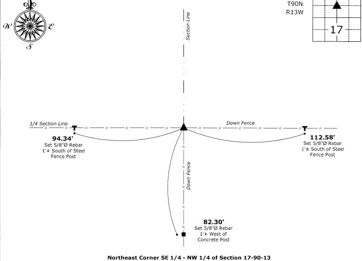
Northeast Corner SE 1/4 - NW 1/4 of Section 17-90-13 Set 5/8"Ø Rebar w/2"Ø Aluminum Cap PLS 22468
