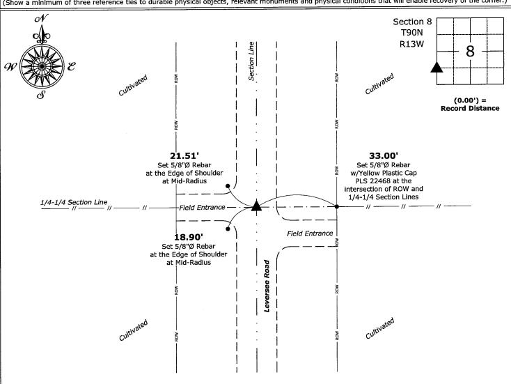
Southwest Corner of the NW 1/4 - SW 1/4 of Section 8-90-13 Set 5/8"Ø Rebar w/2"Ø Aluminum Cap PLS 22468
