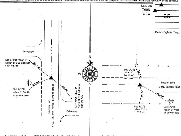
Northwest Corner SW 1/4-NW 1/4 Section 25-90-12 Set MAG nail with stainless steel washer PLS 15525
