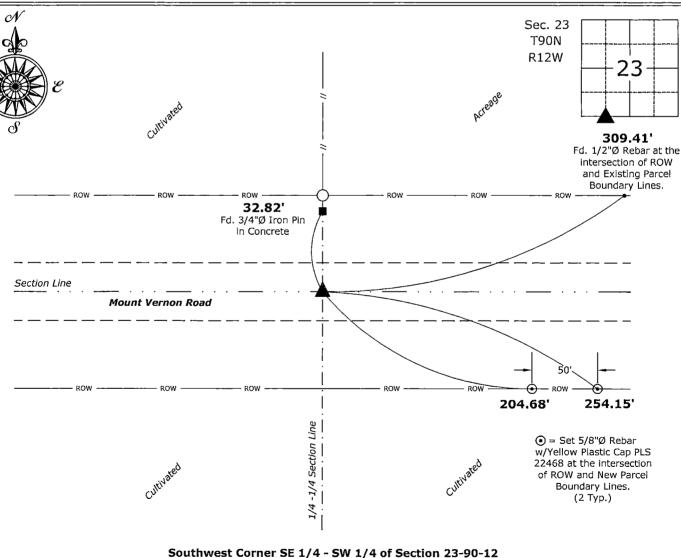
Found 5/8"Ø Rebar, bent. Removed and Reset 5/8"Ø Rebar w/2"Ø Aluminum Cap PLS 22468
