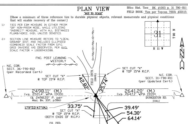
PH.\_PED. -0--SET MAGNAIL W/WASHER CONCRETE @ N.E. FACE FNC. POST @ ±1.0' HT. COR. POST S.P.C., la. N. Zone, USft GATE SET MAGNAIL w/WASHER @ N.E. FACE FNC, POST @ ±1,0' HT, N = 3673555.02FIELD ENTR. E = 5274026.63(GRAVEL) CONVERGENCE = 0° 53' 16" FIELD SURVEY: S.S. & V.S. 7/10/12 (NAD83-NSRS2007 "BHco07", RTK OBS.) PREPARED BY: S.S. & G.T.
