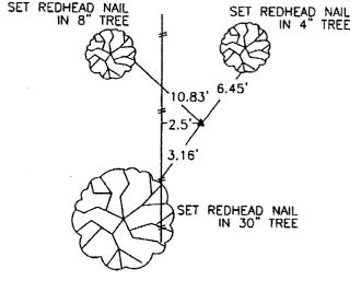
PREVIOUSLY RECORDED IN BOOK \_\_\_\_\_ PAGE \_\_\_\_ MONUMENT DESCRIPTION AND HOW ESTABLISHED \_\_\_ FOUND SPIKE IN E. BENNINGTON RD LOCATION FIT COUNTY ENGINEER TIES AND CHAINING NOTES SET 1/2" REBAR YPC 9647 IN SAME LOCATION AFTER FURTHER SEARCHING
