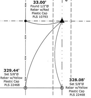
Northeast Corner SE 1/4 - NE 1/4 of Section 11-90-11 Found 1/2"Ø Rebar w/2"Ø Aluminum Cap PLS 10793
