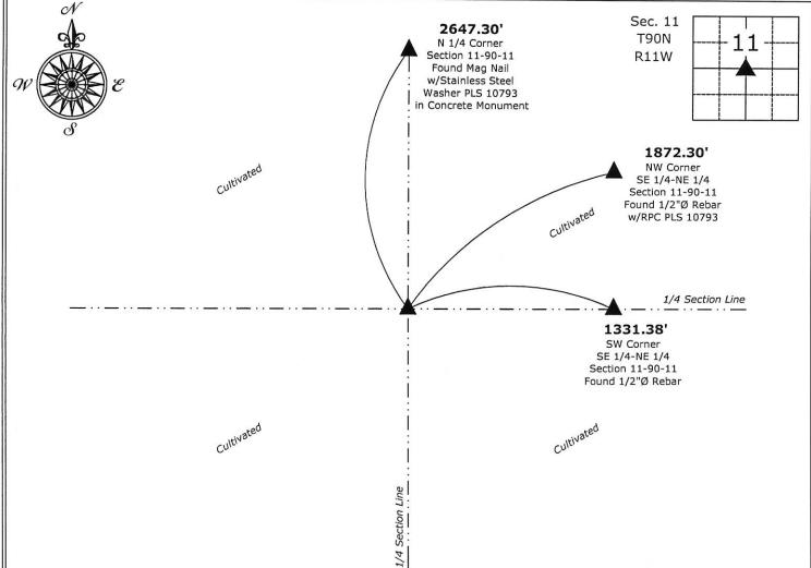
Center of Section 11-90-11 Found 1/2"Ø Rebar w/Red Plastic Cap PLS 10793
