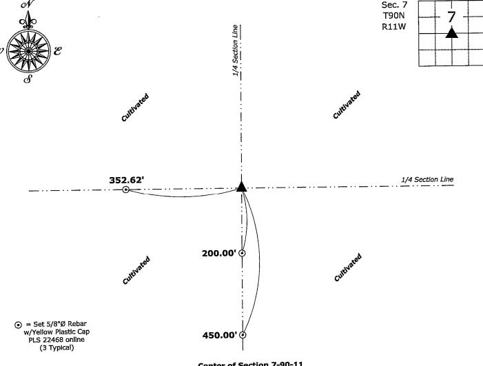
Center of Section 7-90-11 Set 5/8"Ø Rebar w/2"Ø Aluminum Cap PLS 22468
