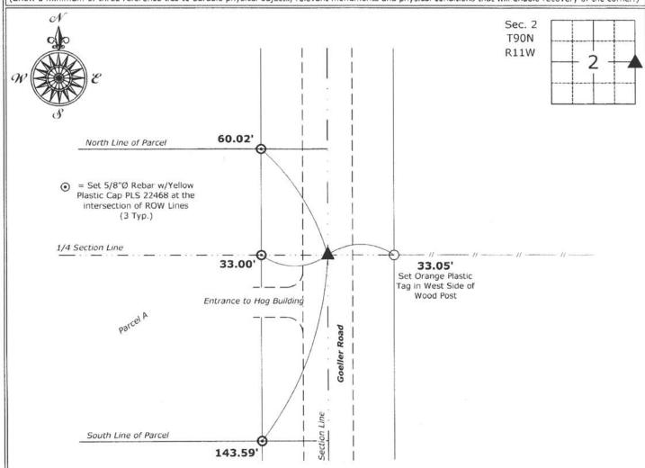
East 1/4 Corner of Section 2-90-11 Set 5/8"Ø Rebar w/2"Ø Aluminum Cap PLS 22468
