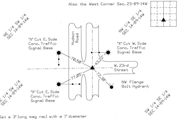
Set a 3" long mag nail with a 1" diameter head stamped Survey Marker.
