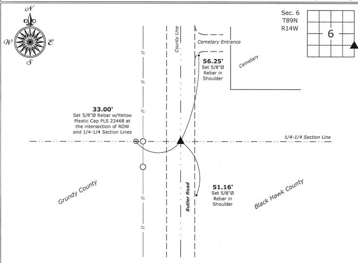
Northwest Corner SW 1/4 - SW 1/4 of Section 6-89-14 Set 5/8"Ø rebar w/2"Ø aluminum cap PLS 22468
