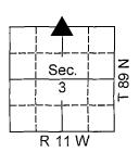
North 1/4 Corner Section 3-89-11 Found #6 Rebar 4" Below Road Surface
