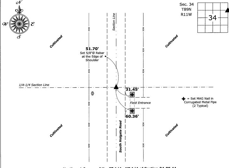
Northeast Corner of the SE 1/4 - NE 1/4 of Section 34-89-11 Set 5/8"Ø Rebar w/2"Ø Aluminum Cap PLS 22468
