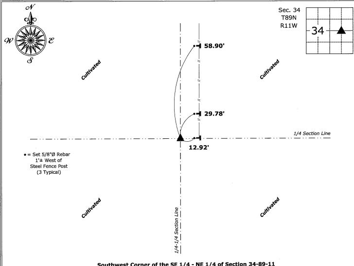
Southwest Corner of the SE 1/4 - NE 1/4 of Section 34-89-11 Set 5/8"Ø Rebar w/2"Ø Aluminum Cap PLS 22468
