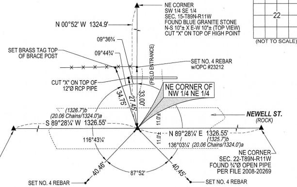
N 1/4 CORNER SEC. 22-T89N-R11W FOUND STANDARD CONCRETE MONUMENT w/BRASS CAP (2.3'± DEEP) SET NO. 4 REBAR
