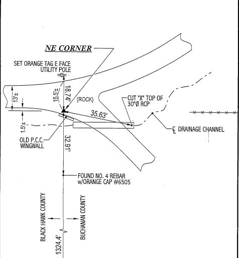
12 BLACK HAWK COUNTY 14'±  $2.5' \pm$ CORNER OF SE 1/4 NE (GRASS) 673.0' (673.9')(CULTIVATED FIELD) (CULTIVATED FIFLD) 50 (GRASS) FOUND NO. 4 REBAR w/ORANGE CAP #6505 (CULTIVATED FIELD) SET ORANGE TAG NW FACE UTILITY POLE E 1/4 CORNER
