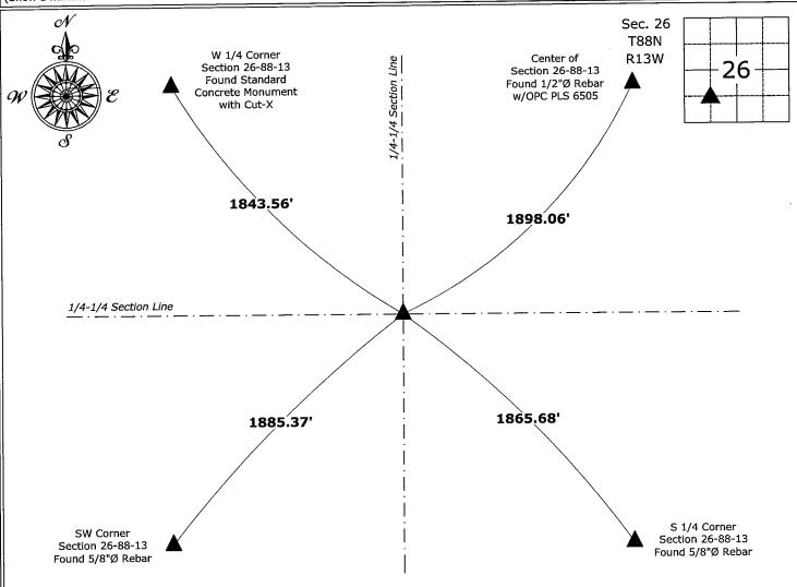
Northeast Corner of the SW 1/4 - SW 1/4 of Section 26-88-13 Set 5/8"Ø Rebar w/2"Ø Aluminum Cap PLS 22468
