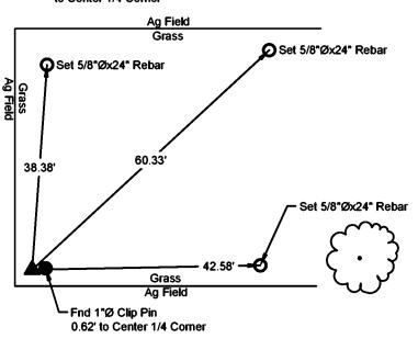
South 1/4 Comer Section 9-T88N-R13W Fnd 1/2Ø Rebar w/Red Cap #16775 per File No. 2016-9568 N00°26'30"W 2649.98' to Center 1/4 Corner
