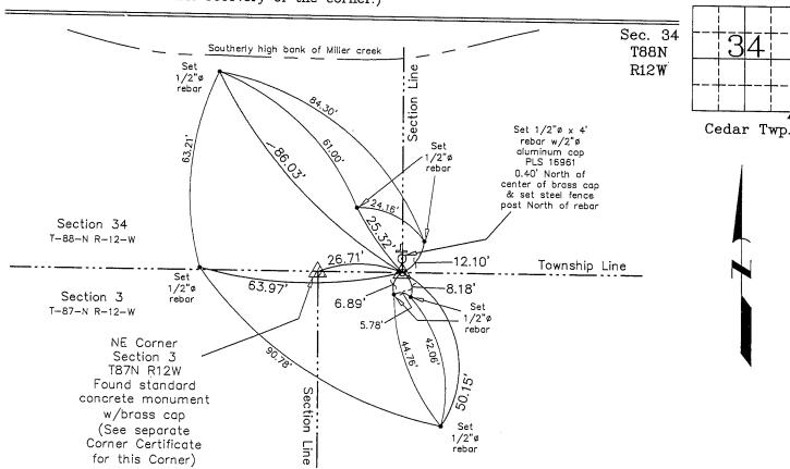
SE Corner Section 34 T88N R12W Found concrete monument w/brass cap, 6" deep. Set 1/2"ø x 4' rebar w/2"ø aluminum cap PLS 16961 at North side of monument, 0.40' from center of brass cap.
