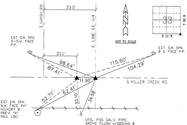
UTIL. FND. GALV. PIPE. DROVE FLUSH w/GROUND @ EST. 42" L. X 5/8" RBR IN CNTR. w/CARSONITE POST.
