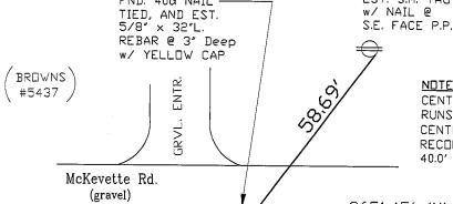
CENTERLINE OF ROAD RUNS 6.5'-7.0' NORTH OF CENTER E. 1/4 LINE, AT A RECORD 26.0' TO S. ROW AND 40.0' TO N. ROW (66' R.O.W.)
