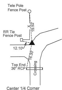
Center 1/4 Corner Section 20-88-12 Set 1/2" rebar w/cap #17344
