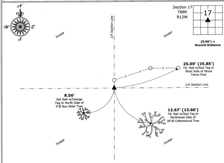
Center of Section 17-88-12 Found 3/4"Ø Iron Pipe w/Orange Plastic Cap PLS 6505
