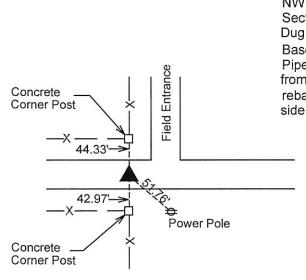
NW Corner Section 25-88-11 Dug and found SCM Base 18" deep with 2" Dia. Pipe 30-1/2" long laid over from WPA notes. Set 1/2" rebar at middle on north side of SCM base, 4" deep.
