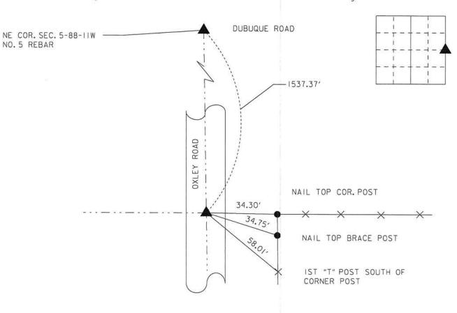
EAST CORNER OF SECTION 5-88-11W FOUND 6" SPIKE 6" DEEP IN LINE WITH FENCE GOING TO THE EAST. RESET 24" NO. 4 REBAR 6" DEEP.
