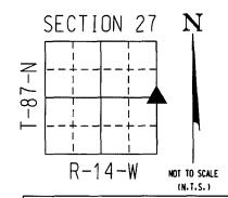
COORDINATE VALUE WAS ESTABLISHED UTILIZING NAD83 (2011)(EPOCH 2010) DATUM USING THE IOWA REGIONAL COORDINATE SYSTEM ZONE 5 PROJECTION IN U.S. SURVEY FEET
