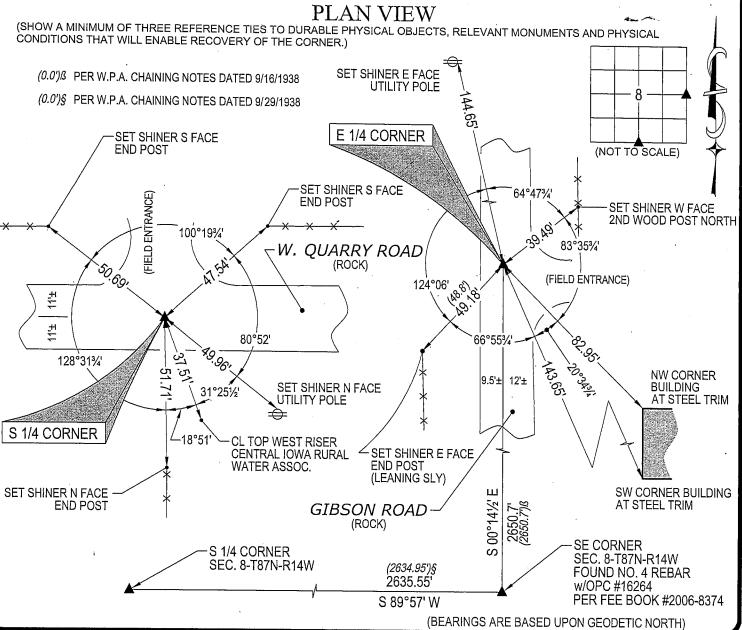
HELLAND ENGINEERING & SURVEYING, LTD. SHINER = 8D NAIL & 1 15/16"Ø METAL SHINER OPC = PLASTIC CAP (O=ORANGE, R=RED, Y=YELLOW)
