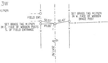
SW CORNER SEC. 34-T87N-R13W FOUND NAIL WITH 3/8" DIAMETER HEAD
