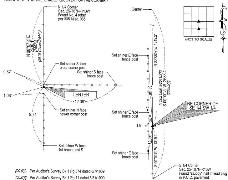
(Bearings are based upon Geodetic North)
