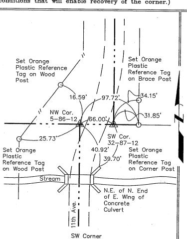
Sec. 32 T87N R12W Big Creek Twp. Set 1/2"ø S 1/4 Cor. 32-87-12 Rebar with Red Plastic Cap 43.404 PLS 7060 N 1/4 Cor 51.15 -86-12 00 -52.04 42.72'-1.21 Sèt Orange Set Orange Plastic Plastic Reference Reference Tag Tag on on Wood Post Corner Post
