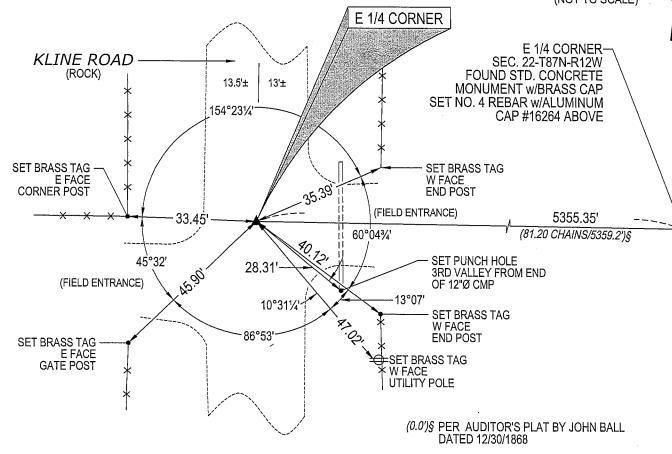
(BEARINGS ARE ASSUMED) HELLAND ENGINEERING & SURVEYING, LTD. SHINER = 8D NAIL & 1 5/16"Ø METAL SHINER
