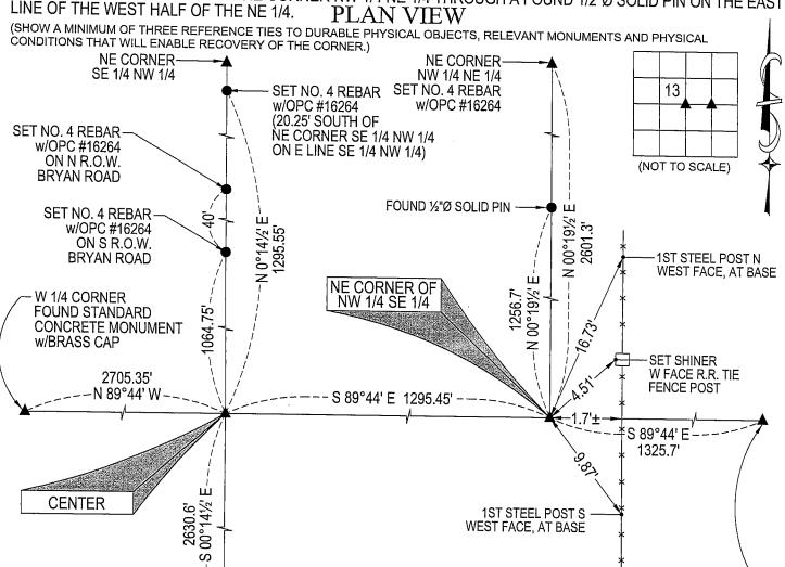
(BEARINGS ARE BASED UPON GEODETIC NORTH) HELLAND ENGINEERING & SURVEYING, LTD.
