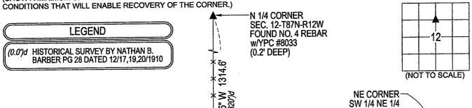
00°03'55" SEC. 12-T87N-R12W FOUND YELLOW GRANITE STONE (5"±N-Sx10"E-W TOP VIEW) **NE CORNER OF** (1.2' DEEP) CUT "X" ON TOP SE 1/4 NW 1/4  $\bar{-}$ 11.71
