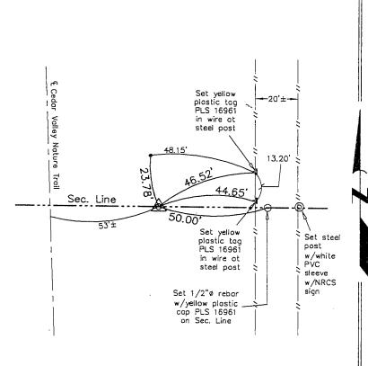
N 1/4 Corner Section 10 T87N R12W Found 1/2"ø rebar w/yellow plastic cap 7034
