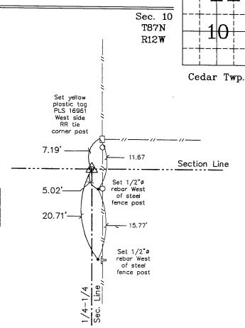
NW Corner NE 1/4 - NE 1/4 Section 10 T87N R12W Found 1/2"ø rebar
