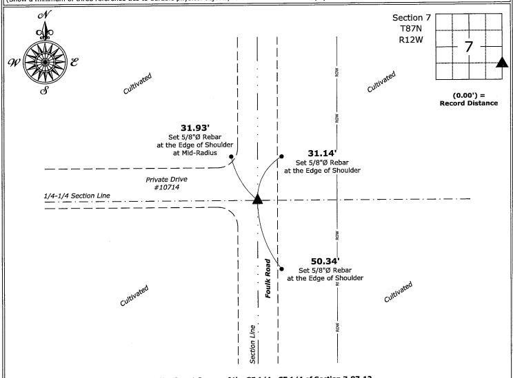
Northeast Corner of the SE 1/4 - SE 1/4 of Section 7-87-12 Set 5/8"Ø Rebar w/2"Ø Aluminum Cap PLS 22468
