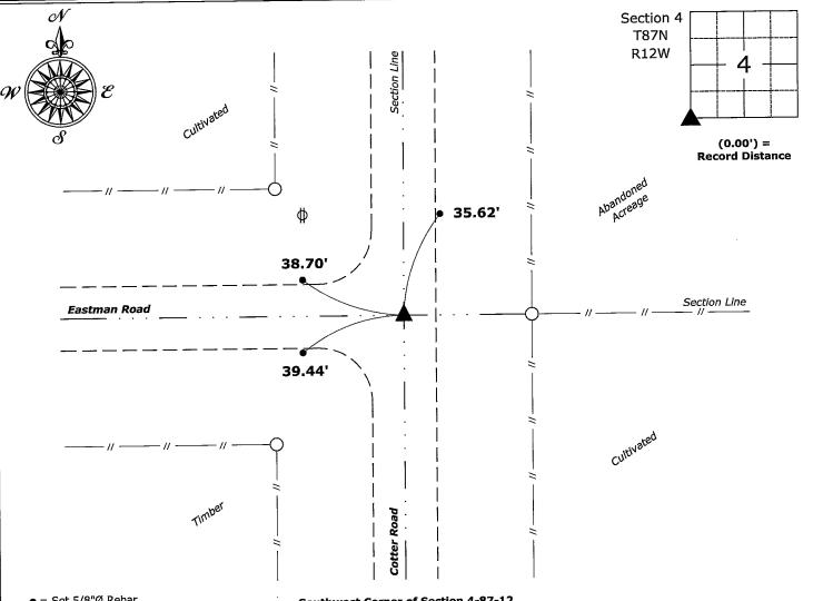
■ = Set 5/8"Ø Rebar at the Edge of Shoulder Inline with Power Pole (3 Typical)
