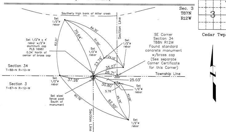
NE Corner Section 3 T87N R12W Found concrete monument w/brass cap, 6" deep. Set 1/2"ø x 4' rebar w/2"ø aluminum cap PLS 16961 at North side of monument, 0.34' from center of brass cap.
