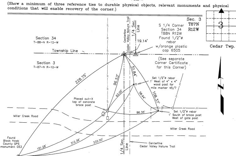
N 1/4 Corner Section 3 T87N R12W Set 1/2"ø rebar w/2"ø aluminum cap PLS 16961
