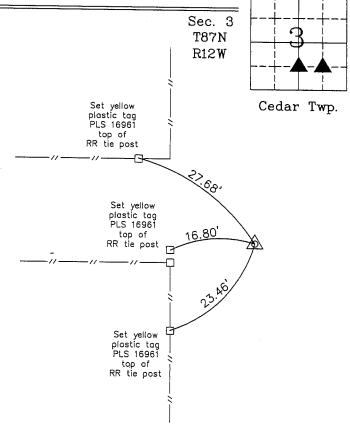
SE Corner NW 1/4 - SE 1/4 Section 3 T87N R12W Set 1/2"ø rebar w/2"ø aluminum cap PLS 16961
