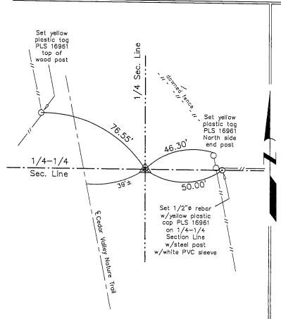
SW Corner NW 1/4 - SE 1/4 Section 3 T87N R12W Set 1/2"ø rebar w/2"ø aluminum cap PLS 16961
