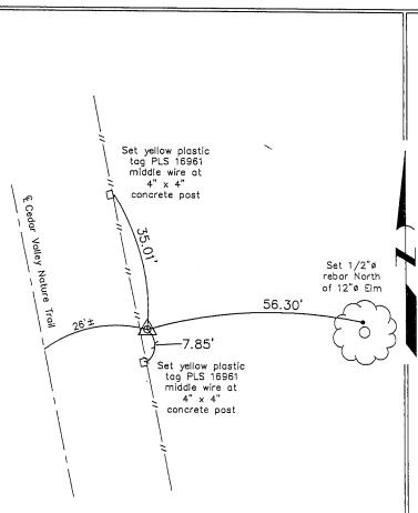
Center of Section 3 T87N R12W Set 1/2"ø rebar w/2"ø aluminum cap PLS 16961
