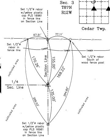
E 1/4 Corner Section 3 T87N R12W Set 1/2"ø rebar w/2"ø aluminum cap PLS 16961, 18" deep
