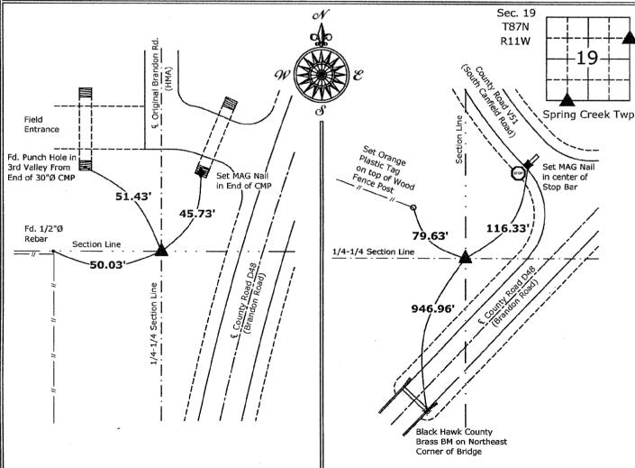
1.) Southwest Corner SE 1/4-SW 1/4 Section 19-87-11 Set 5/8"Ø rebar w/2"Ø aluminum cap PLS 19211
